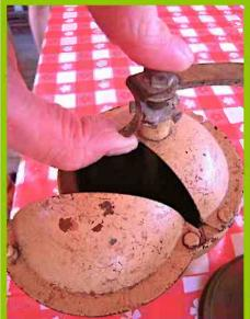
Peugeot coffee mills were renowned for their "burred helical" grinder. The grind can be adjusted by turning the thumb screw below the crank handle. Its best turned slow and steady so as not to heat the mechanism and release volatile oils before the coffee is brewed. Aha!
